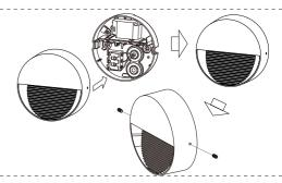
Fix the cover with side cap screws.
