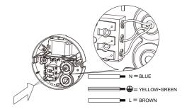
Connect AC wires correspondingly.
